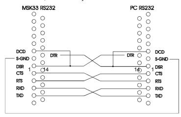
of the MSK 33 works faster, if the handshake operation is activated (especially, if no modem is connected). The MSK 33 first answers without handshake after the entry of a RE-TURN on the PC.
